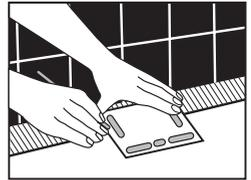
Put the tile to be cut upside down in gap near the wall. Mark where to be cut. Allow for spacing.
