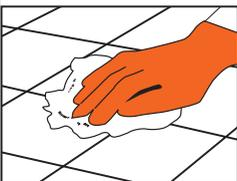
Clean off grout with a damp sponge and when grout lines are dry polish off with a soft cloth.
