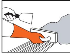
Starting at the centre of the room spread a square metre of adhesive using a notched trowel and work to walls.
